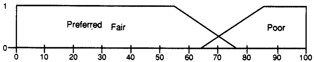
Fig. 21d. Membership functions for depth for the Surfactant/Polymer Method.
